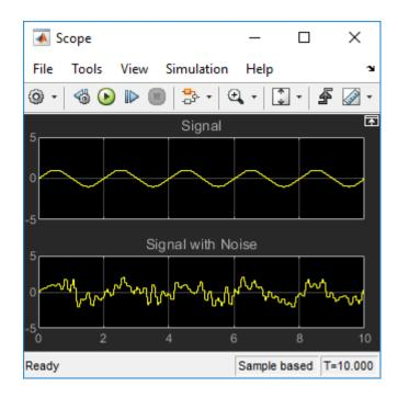
You have now built a digital filter and used it to model the presence of colored noise in your signal. This is analogous to modeling the low frequency noise reaching the microphone in the cockpit of the aircraft. Now that you have added noise to your system, you can experiment with methods to eliminate it.
