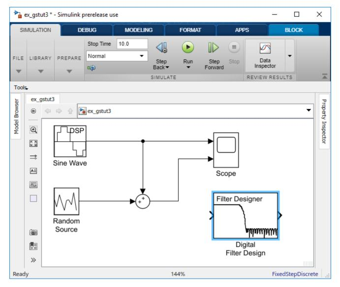
Set the Digital Filter Design block parameters to design a lowpass filter and create low frequency noise. Open the block parameters dialog box by double-clicking the block. Set the parameters as follows:
