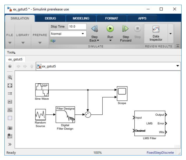
Set the LMS Filter block parameters to model the output of the Digital Filter Design block. Open the LMS Filter dialog box by double-clicking the block. Set and apply the block parameters as follows:
