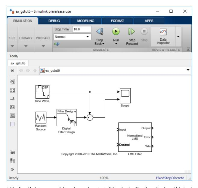
Add a Sum block to your model to subtract the output of the adaptive filter from the sinusoidal signal with low frequency noise. From the Simulink fallback for  $tm_simulink$  Math Operations library, drag a Sum block into your model. Open the Sum dialog box by double-clicking this block. Change the **List** of signs parameter to |+- and then click OK.
